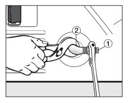
■ Install a <sup>3</sup>/<sub>8</sub>" flare union adapter, ①, to the female elbow, ②.
